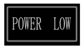
When the radio detects that the power supply voltage is below 10V, "POWER LOW" will be displayed on the radio LCD.
